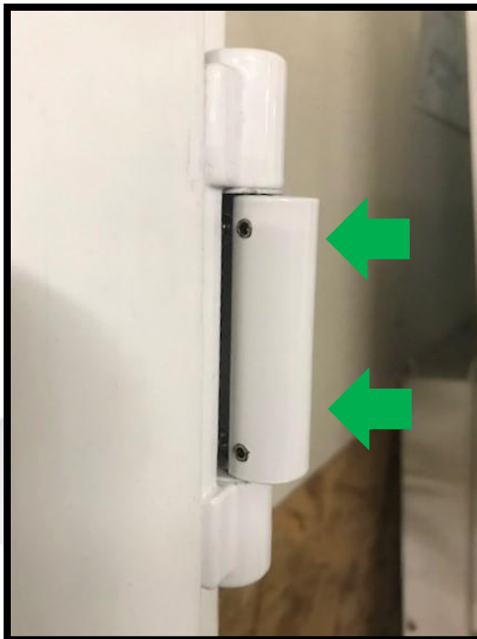
Figure 23: Re-installing the Cover Plate
