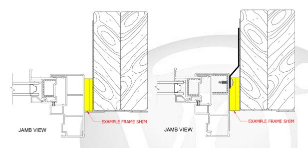
B) Additional shims may be required for support and squaring at the top of the jambs. It is the installers' responsibility to address any rough opening framing issues during installation.
